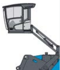
Cab system hydraulically adjustable
