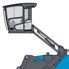
Cab system hydraulically adjustable
